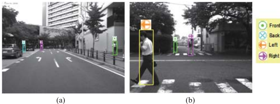
Fig. 3 Results of the pedestrian detection. Rectangles show the detected pedestrian and symbols on the top of the rectangles show the estimated direction by our proposed method.
