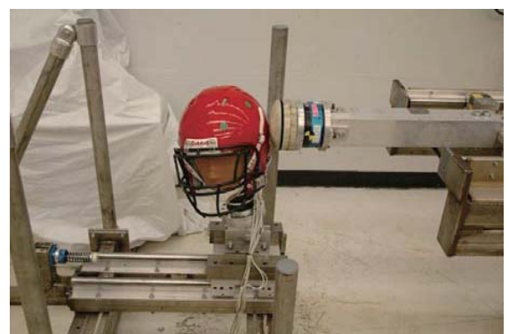
Fig. 3 Pneumatic linear impactor and helmeted Hybrid III head mounted on the linear slide table.
