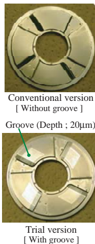
Fig. 4 Test peaces of compliant foil thrust bearing.
