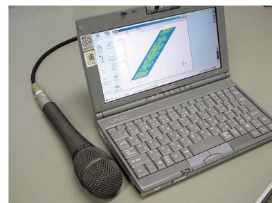
Fig. 3 Realtime visualization system for vehicle sound color.
