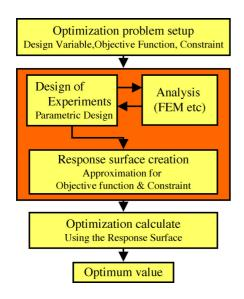
Fig. 2 Response Surface Methodology (RSM).
