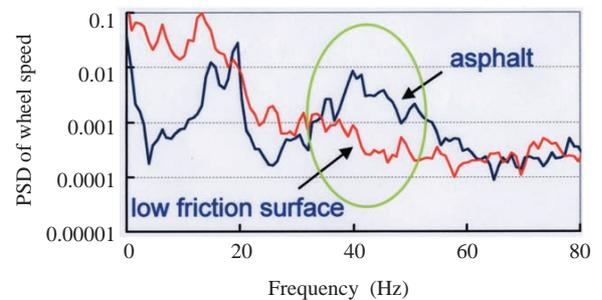
Fig. 1 PSD of wheel angular velocity.
