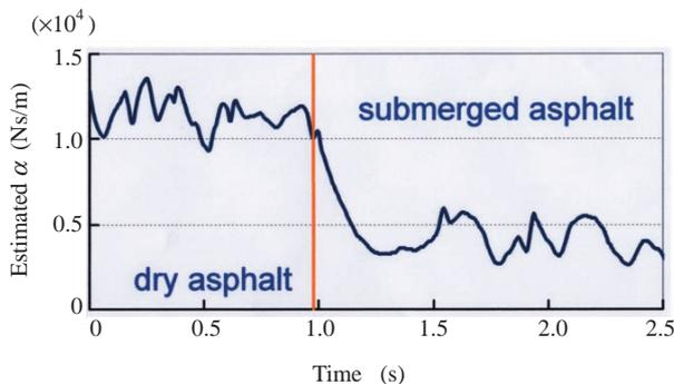
**Fig. 10** Estimation result for hydroplaning test.
