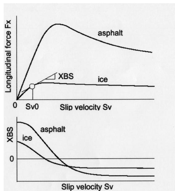
Fig. 2 Longitudinal force and extended braking stiffness.
