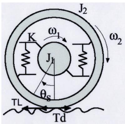
**Fig. 3** Tire vibration model.
