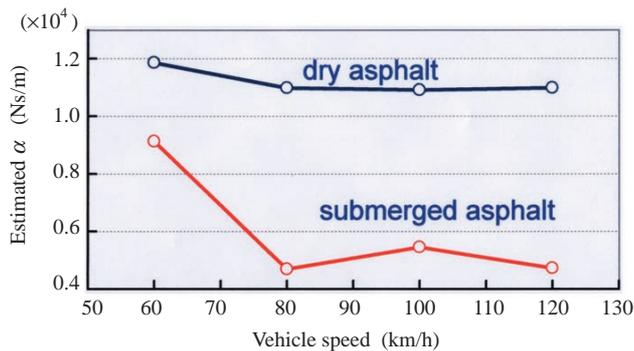
**Fig. 9** Estimated  $\alpha$  at submerged asphalt for each vehicle speed.
