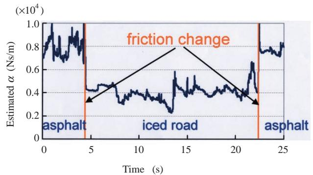
Fig. 8 Estimation result on the iced road.
