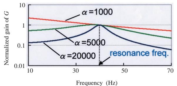
**Fig. 4** Frequency characteristic of  $G(j\omega)$ .
