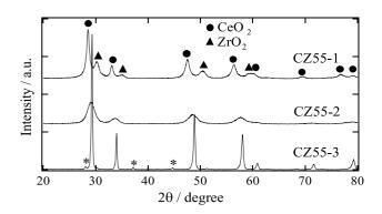
X-Ray diffraction patterns of CeO<sub>2</sub>-ZrO<sub>2</sub> samples having the same composition ratio (Ce/Zr = 1). Small peaks indicated with asterisks are characteristic of  $\kappa$ -Ce<sub>0.5</sub>Zr<sub>0.5</sub>O<sub>2</sub>, and are a reflection of the ordered arrangement of the cations<sup>6)</sup>.
