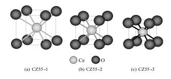
**Fig. 5** Schema illustrating oxygen environment around Ce. The Ce-O bond length gradually shortens in the order CZ55-1 > CZ55-2 > CZ55-3.
