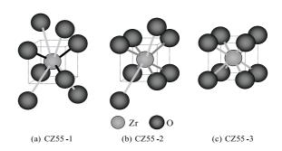
**Fig. 6** Schema illustrating oxygen environment around Zr. In CZ55-1, a pure tetragonal ZrO<sub>2</sub> forms and has two sets of short and long Zr-O bond lengths. In CZ55-2, the Zr-O coordination is, on average, somewhat more centrosymmetric than that in tetragonal ZrO<sub>2</sub>. The configuration of the oxygen around Zr for CZ55-3 has a hightly symmetric 8-fold coordination.
