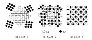
**Fig. 4** Schema illustrating the cation-cation network in the  $CeO_2$ - $ZrO_2$  samples having the same composition (Ce/Zr=1). CZ55-1 consists of pure  $CeO_2$  and  $ZrO_2$ . A  $CeO_2$ - $ZrO_2$  solid solution forms in CZ55-2, but the Ce- and Zr-rich domains still remain. The  $Ce_{0.5}Zr_{0.5}O_2$  solid solution that forms in CZ55-3 is homogeneous at atomic level, possessing an ordered arrangement of Ce and Ce and Ce ions.
