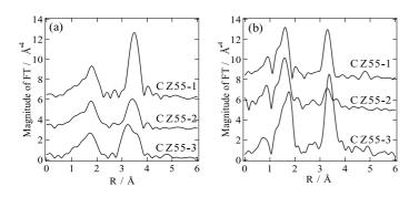
Fig. 2 Fourier-transformed  $\kappa^3 x$  data of (a) Ce K-edge and (b) Zr K-edge EXAFS of CeO<sub>2</sub>-ZrO<sub>2</sub> samples.
