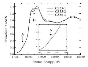
**Fig. 3** Zr K-edge XANES spectra of CeO<sub>2</sub>-ZrO<sub>2</sub> samples.
