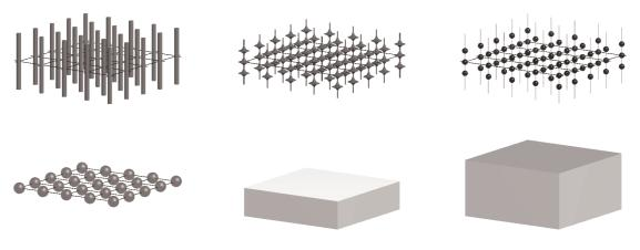
(a) An ideal 2-dim. Crystal (below). r-space consists of rods (above).
