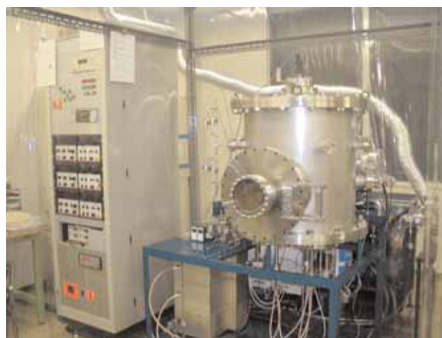
Fig. 3 Photograph of new sputter-coating apparatus with 3 RF-magnetron 4 inch-cathodes in a vacuum chamber (right).
