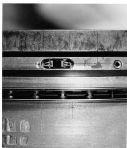
Fig. 3 State of attachment of pressure sensor to piston.
