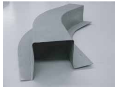
Fig. 11 Photographical view of stamping rail model panel.
