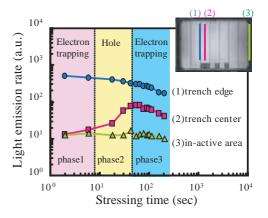
**Fig. 8** Light emission rate of test sample as a function of stressing time under a constant voltage stress (Vg=63V).
