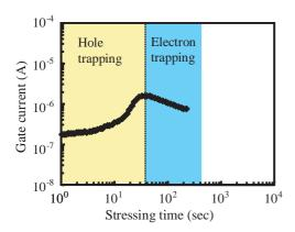
**Fig. 9** Gate current of planar capacitor as a function of stressing time under a constant voltage stress.
