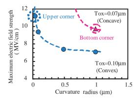
Fig. 6 Simulation results of maximum electrical field strength as a function of curvature radius.
