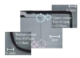
**Fig. 5** Transverse (x-axis) cross-sectional SEM photographs of test sample.
