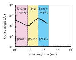
**Fig. 7** Gate current of test sample as a function of stressing time under a constant voltage stress (Vg=63V).
