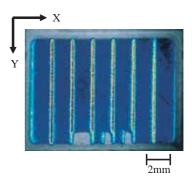
**Fig. 4** Light emission image of test sample. Localized electron injection occurred at the trench edge in the longitudinal direction (y-axis).
