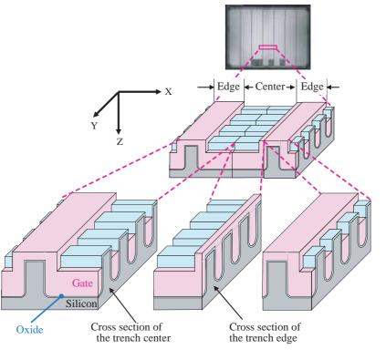
**Fig. 2** Structure of test sample. The trench gate is interconnected at the trench edge in the longitudinal direction (y-axis). The trench gate touches the trench oxide layer at the upper corner of the trench edge.
