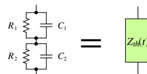
**Fig. 3** Cell of proposed compact thermal model.
