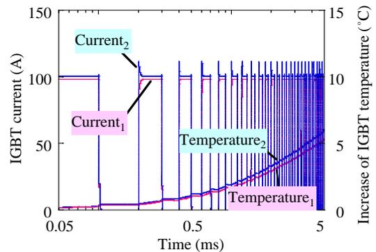
(a) The case of different threshold voltages (IGBT<sub>1</sub>: 6.83 V, IGBT<sub>2</sub>: 6.33 V).
