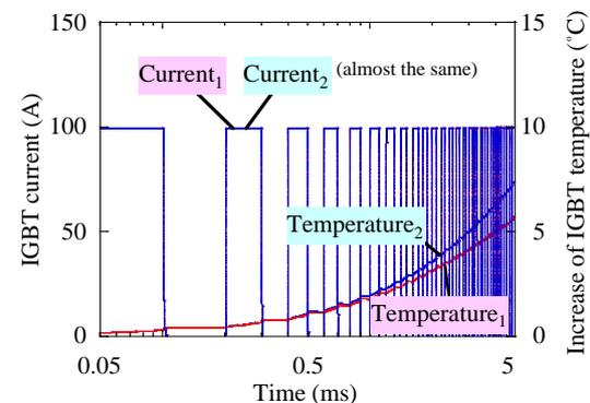
(b) The case of different thermal resistances (IGBT<sub>1</sub>: 0.49 K/W, IGBT<sub>2</sub>: 0.54 K/W).
