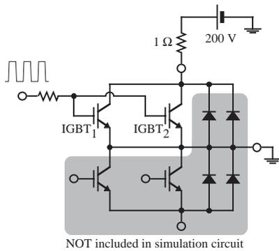
**Fig. 7** Simulation circuit.
