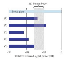
Fig. 8 The measurement result of the reflective intensity of the clothes.
