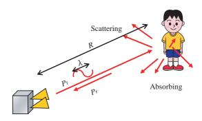
Fig. 1 Radio wave reflective model in pedestrian.
