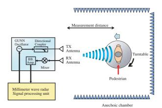
**Fig. 2** Structure of the measurement system.
