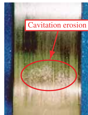
Fig. 2 Cavitation erosion on bearing surface.
