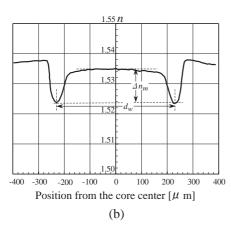
**Fig. 5** Refractive index profile after UV exposure. (a) Interferogram obtained by interference microscopy, (b) calculated refractive index profile.
