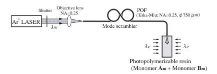
**Fig. 2** Schematic diagram of the experimental set-up used for fabrication of the LISW waveguides.
