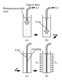
**Fig. 1** Fabrication processes to produce LISW waveguides for use with large-core optical fibers.
