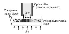
**Fig. 3** Experimental set-up used to investigate refractive index changes induced by photopolymerization.
