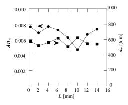
**Fig. 7** The dependence of the maximum refractive index difference  $\Delta n_m$  and the core diameter  $d_w$  on the distance from the fiber tip.
