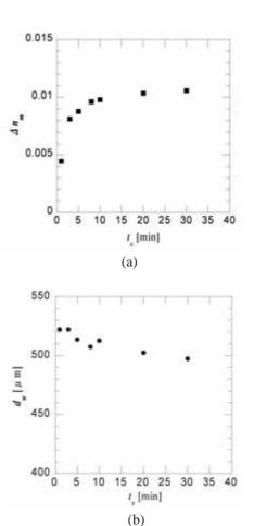
**Fig. 6** Changes in the maximum refractive index difference  $\Delta n_m$  (a) and the core diameter  $d_w$  (b) against the diffusion time  $t_x$ , observed after UV exposure.
