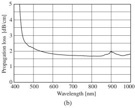
Fig. 8 Loss properties of an LISW optical waveguide measured by a cutback method.
