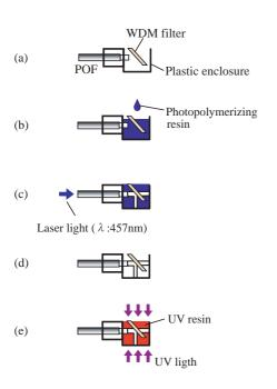
**Fig. 2** Process flow used to fabricate a LISW waveguide module. (a) Setting, (b) Resin for core filling, (c) Core forming, (d) Removal of residual resin, (e) Resin for cladding fill and curing.
