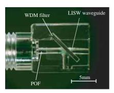
**Fig. 4** Example of the produced LISW waveguide module.
