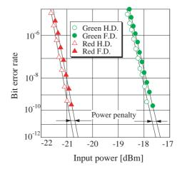
Fig. 5 Results of the BER measurements.
