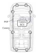
Fig. 6 On-board camera network for vehicles.
