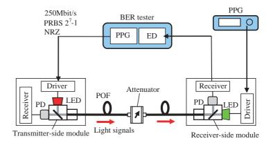
**Fig. 3** Experimental set-up for bit error rate measurements.
