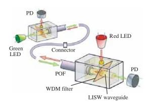
**Fig. 1** Diagram of a bi-directional single POF communication system using LISW waveguide modules.
