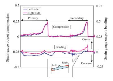
Fig. 9 Measurement result of element width direction strain.  $(N_{in}=1000$ rpm, without load, speed ratio=0.7)
