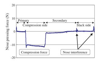
Fig. 7 Measurement result of element nose strain. ( $N_{in}$ =500rpm,  $T_{in}$ =150Nm, speed ratio=2.4)
