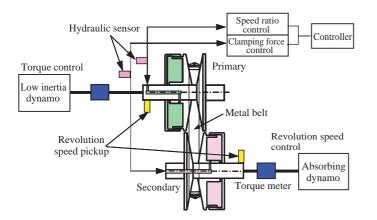
Fig. 4 Schematic of test apparatus.
