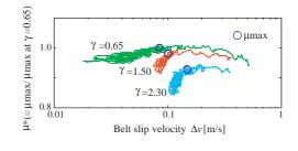
Fig. 13 Relation between slip velocity and belt  $\mu$ . (N<sub>in</sub>=1000rpm, T<sub>in</sub>=100Nm)
