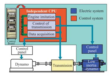
Fig. 1 Dynamo control system.
