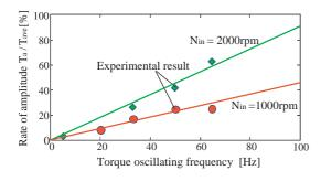
Fig. 15 Ratio of vibration amplitude to the average torque at macro slip occurrence.  $(T_{ave} = 100Nm, speed ratio = 0.65)$
