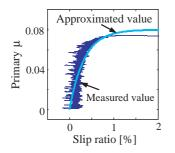
**Fig. 17** Result of approximation of belt  $\mu$ .
