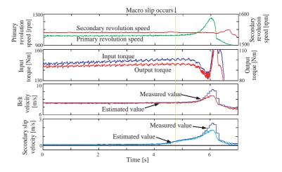
Fig. 18 Result of estimation of belt velocity and belt slip velocity (using bench data).
