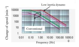
Fig. 3 Speed response of low inertia dynamo.
