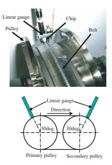
Fig. 10 Pitch radius measurement device.
