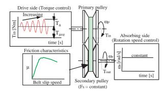
Fig. 14 Method to investigate belt slip by input torque fluctuations.
