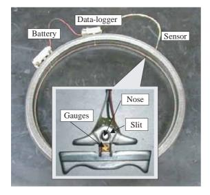
Fig. 6 Nose load sensor and data-logger system.
