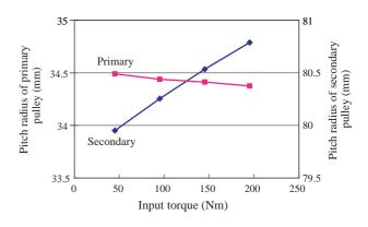
Fig. 11 Measurement result of pitch radius. (N<sub>in</sub>=1000rpm, speed ratio=2.4)
