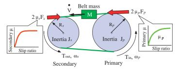
Fig. 16 Model based on belt velocity estimation.
