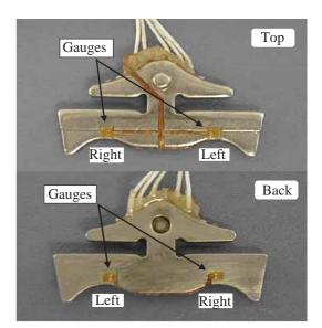
Fig. 8 Width direction load sensor.
