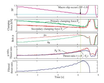
Fig. 19 Time chart of belt  $\mu$  and  $\mu$  ratio around macro slip occurrence.
