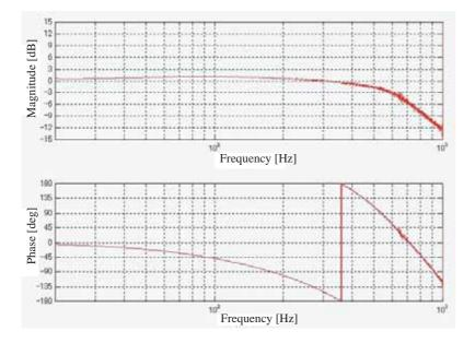
Fig. 2 Torque response of low inertia dynamo.
