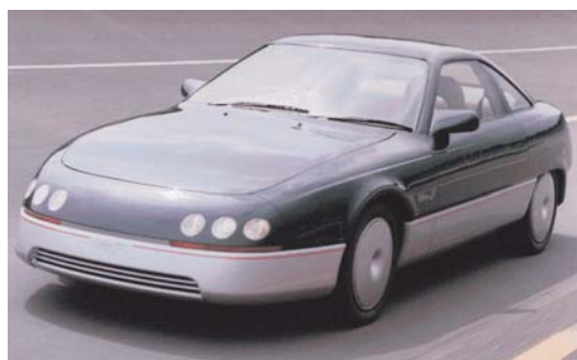
Fig. 4 TOYOTA GTV passenger car powered by a GT41 gas turbine.
