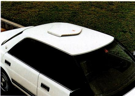
Photo. 2 Phased array antenna with radome mounted on car roof.
