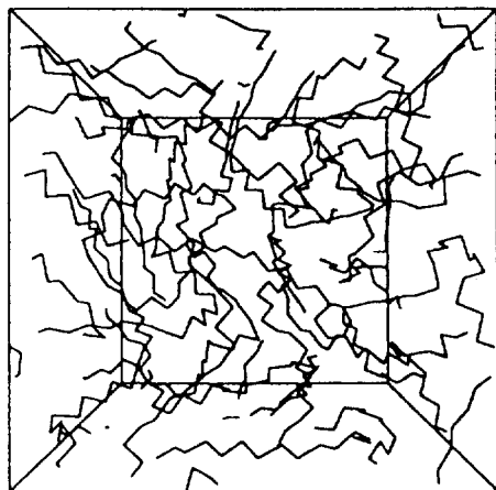
Fig. 7 Two dimensional projection of the MD cell. The length of edges of the cell is about 2.5 nm. 38)
