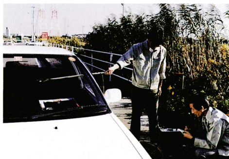
Fig. 23 Photograph of on-site measuring of ELF field in car under high voltage power lines.
