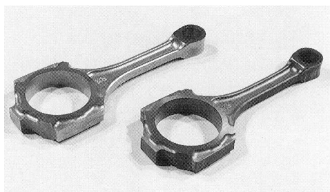
Fig. 26 Trial products of the new BE Ti-6Al-4V alloy (left) and the developed 10vol.%TiB/Ti-6Al-4V MMC (right).
