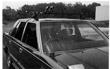
Fig. 9 Setting of a conventional video camera and the developed vision sensor onto the car for the experiments.
