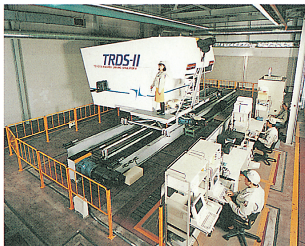
Fig. 10 Experimental scene of 2 DOF driving simulator.
