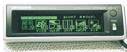
Fig. 21 Photograph of FM multiplex receiver with an organic EL display.
