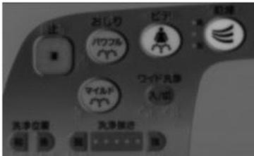
Fig. 10 Simulated image of control panel with illuminated buttons( age60, 100 lux).
