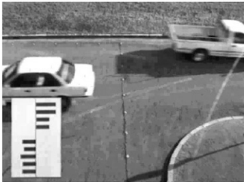
Fig. 9 A result of vehicle detection on a road with the prototype sensor.
