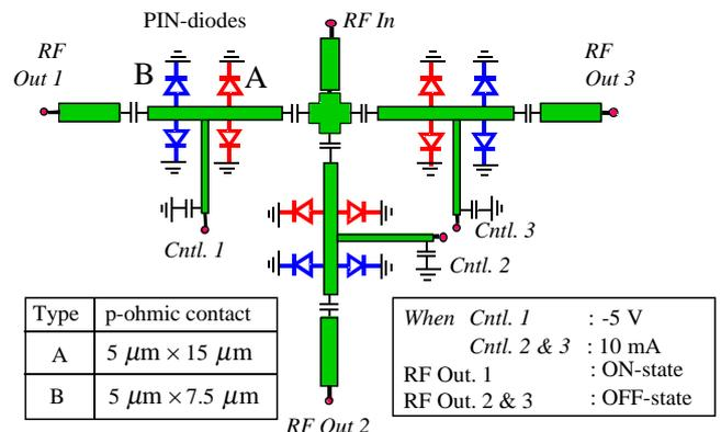
**Fig. 5** Schematic diagram of the SP3T switch circuit.
