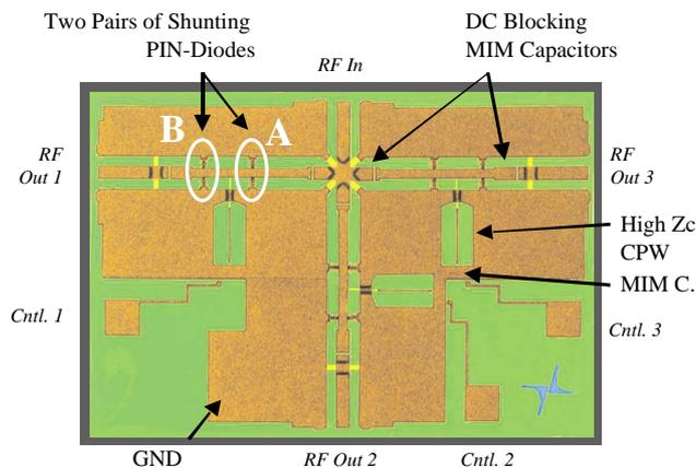
**Fig. 4** Photograph of a fabricated 76-77 GHz double-shunted SP3T GaAs PIN switch MMIC. The actual chip size is  $2.2\ \text{mm} \times 1.4\ \text{mm}$  ( $1.85\ \text{mm} \times 1.2\ \text{mm}$  in effectiveness).
