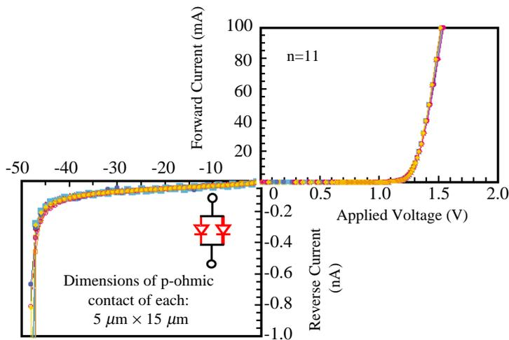
**Fig. 3** I-V characteristics of the parallel pair PIN-diodes.
