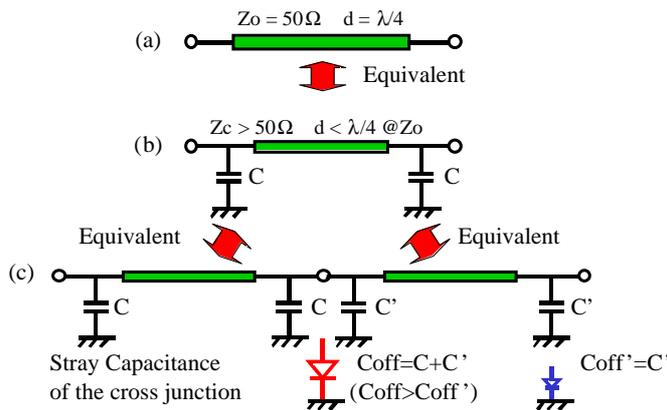
**Fig. 7** Equivalent circuits for the switch arm in the ON-state. (a) fundamentals (b) equivalent transmission line to the fundamentals (c) switch output arm in the ON-state that has been designed to be a series of two equivalent transmission lines.
