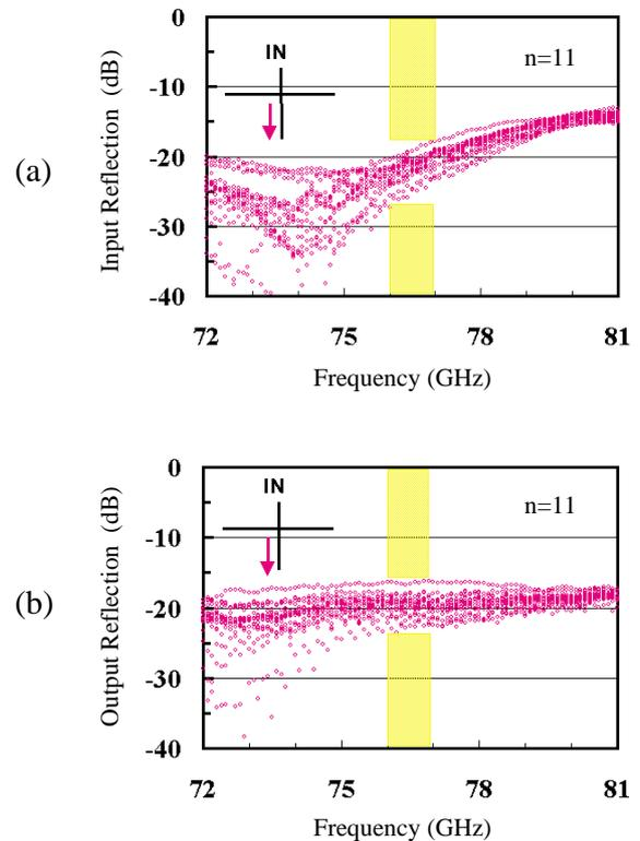
**Fig. 9** Reflection properties of the fabricated SP3T switch. (a) Input reflection when the straight arm is in the ON-state. (b) Output reflection of the straight arm being in the ON-state.
