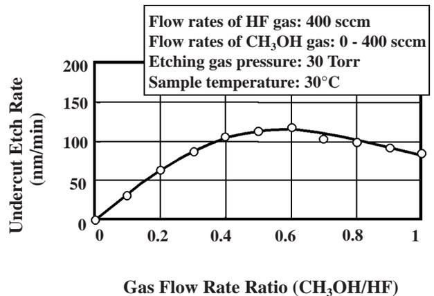
**Fig. 5** Dependence of the undercut etch rate on gas flow rate ratio ( $\text{CH}_3\text{OH}/\text{HF}$ ).
