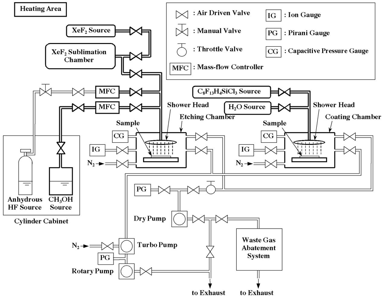
**Fig. 2** A schematic of the micromachining system.
