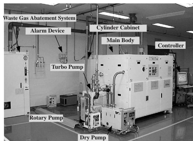
**Fig. 1** A photograph of the micromachining system.
