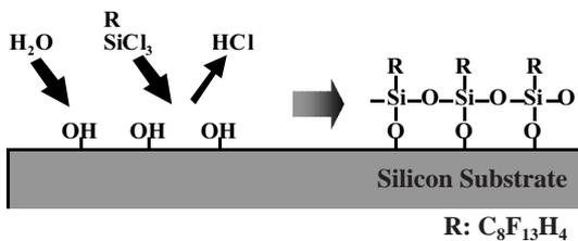
**Fig. 8** A schematic of the silanization reaction.
