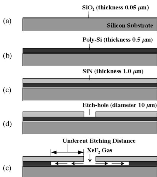
**Fig. 6** Process sequence for fabrication of Poly-Si sacrificial layer etching samples.
