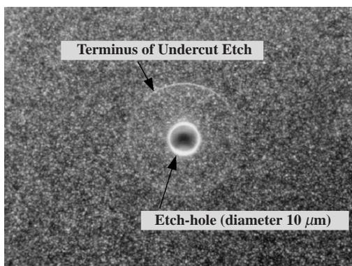
**Fig. 4** A top view photomicrograph of an etched  $\text{SiO}_2$  sacrificial layer.
