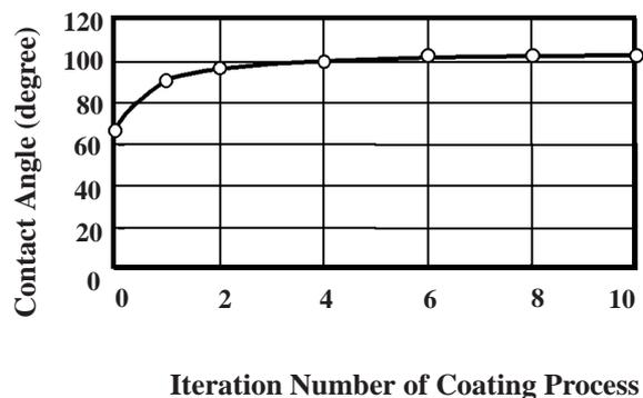
**Fig. 10** Water contact angles of silicon substrates treated by the silanization coating.
