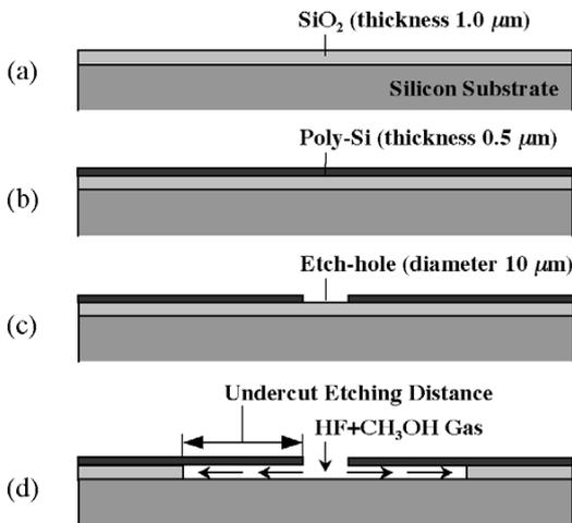
**Fig. 3** Process sequence for fabrication of an  $\text{SiO}_2$  sacrificial layer etching sample.
