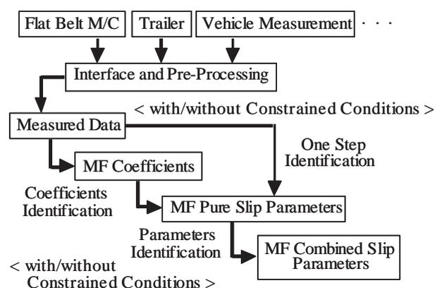
**Fig. 1** Structure of tire model identification system.
