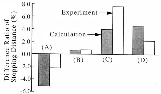
**Fig. 5** Comparison of stopping distance between calculation and experiments.
