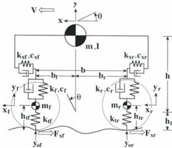
**Fig. 4** Vehicle model and symbol notation.
