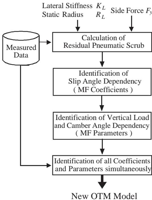
Fig. 6 Procedure of identification of New OTM Model.
