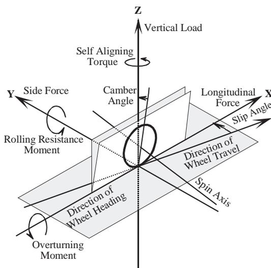
**Fig. 1** The tire coordinate system.
