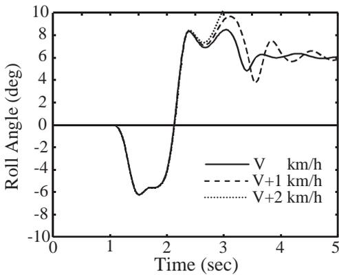
**Fig. 9** The response of roll angle.
