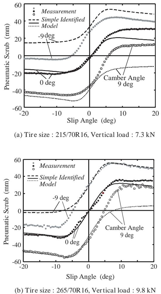
Fig. 4 Comparison of pneumatic scrub between measurement and Simple Identified Model.
