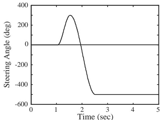
Fig. 8 The steering angle input for vehicle simulation.
