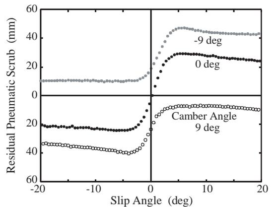
(a) Tire size : 215/70R16, Vertical load : 7.3 kN
