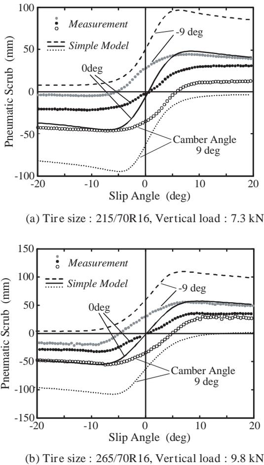
Fig. 3 Comparison of pneumatic scrub between measurement and Simple Model.
