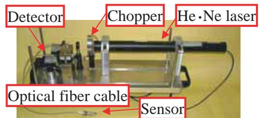
**Fig. 5** Photograph of the developed instrument.
