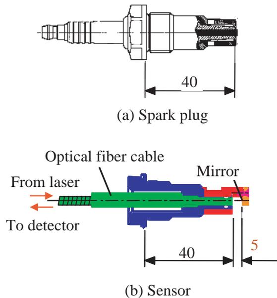
**Fig. 4** Structure of spark plug and sensor.
