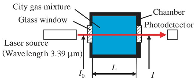
**Fig. 3** Method applied the principle of infrared absorption.
