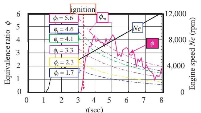
**Fig. 7** Measurement of equivalence ratio and engine speed (diffusion).
