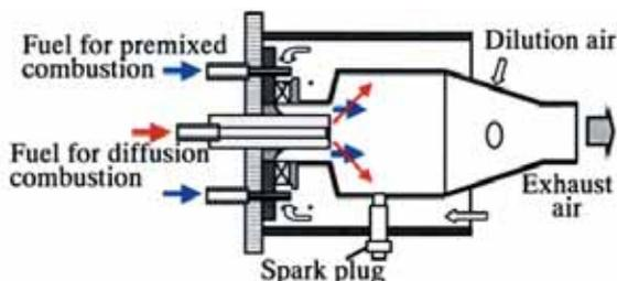
Fig. 1 Structure of TLP combustor.
