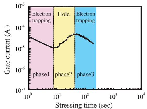
**Fig. 7** Gate current of test sample as a function of stressing time under a constant voltage stress ( $V_g=63V$ ).
