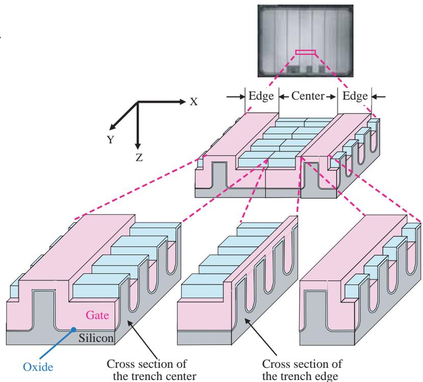
**Fig. 2** Structure of test sample. The trench gate is interconnected at the trench edge in the longitudinal direction (y-axis). The trench gate touches the trench oxide layer at the upper corner of the trench edge.
