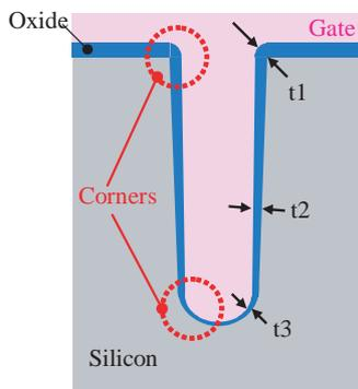
**Fig. 1** Schematic cross-sectional view of a trench gate structure.
