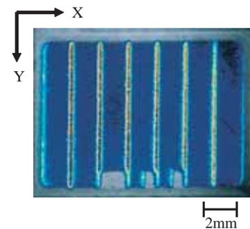
**Fig. 4** Light emission image of test sample. Localized electron injection occurred at the trench edge in the longitudinal direction (y-axis).
