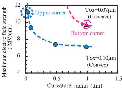
**Fig. 6** Simulation results of maximum electrical field strength as a function of curvature radius. The symbol ● and ▲ in the dotted circles indicate the data at the upper corner and the bottom corner, respectively (see Fig. 5).
