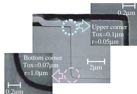
**Fig. 5** Transverse (x-axis) cross-sectional SEM photographs of test sample.
