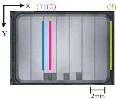
**Fig. 3** Three windows for measuring light emission rate. These windows were used to obtain the distribution of electron injection: 1) the edge of a trench gate, 2) the center of a trench gate, 3) the in-active area, for monitoring the noise level.
