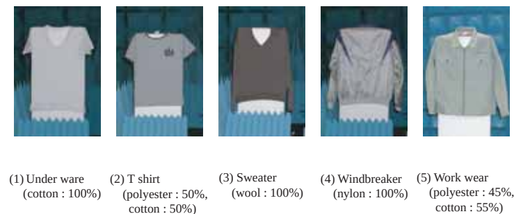
Fig. 7 Five difference kinds of clothes for the measurement of the reflective intensity of the clothes.
