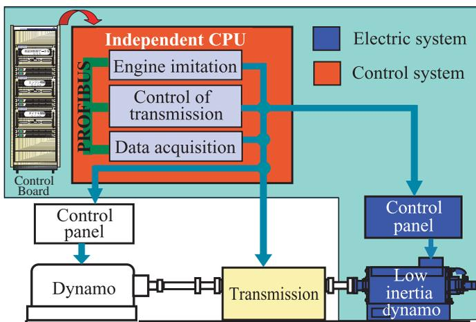
**Fig. 1** Dynamo control system.
