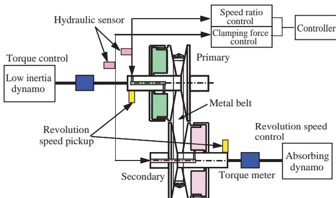
Fig. 4 Schematic of test apparatus.
