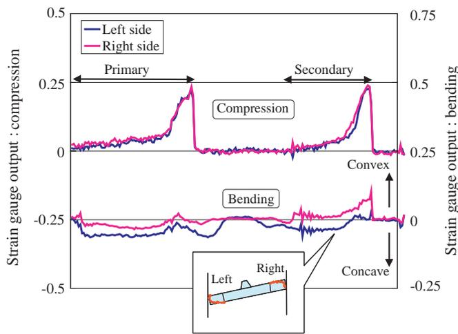
Fig. 9 Measurement result of element width direction strain. ( $N_{in}=1000\text{rpm}$ , without load, speed ratio=0.7)
