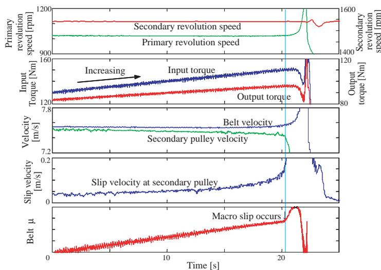
Fig. 12 Measurement result of static belt  $\mu$ . (speed ratio=0.65,  $N_{in}$ =1000rpm)
