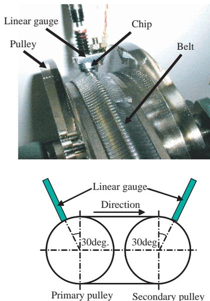
Fig. 10 Pitch radius measurement device.
