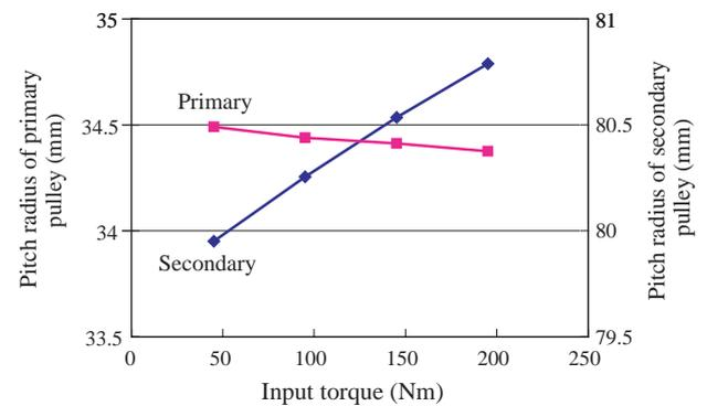
Fig. 11 Measurement result of pitch radius. ( $N_{in}=1000\text{rpm}$ , speed ratio=2.4)
