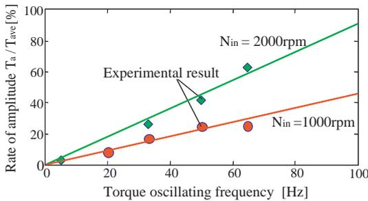
**Fig. 15** Ratio of vibration amplitude to the average torque at macro slip occurrence. (T<sub>ave</sub> = 100Nm, speed ratio = 0.65)
