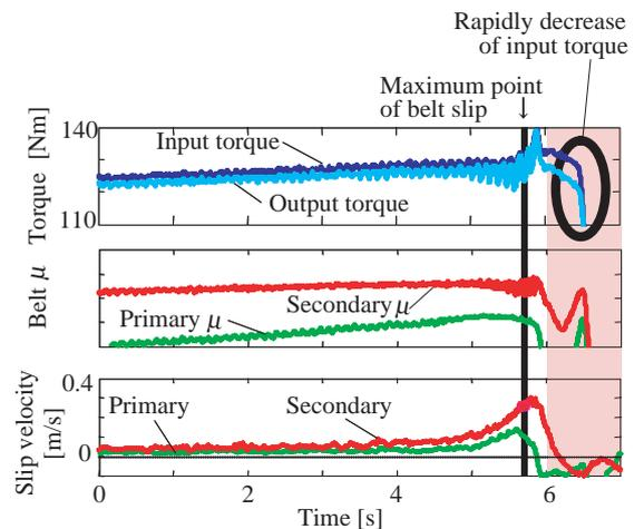
Fig. 5 Friction coefficient at a belt slip limit.
