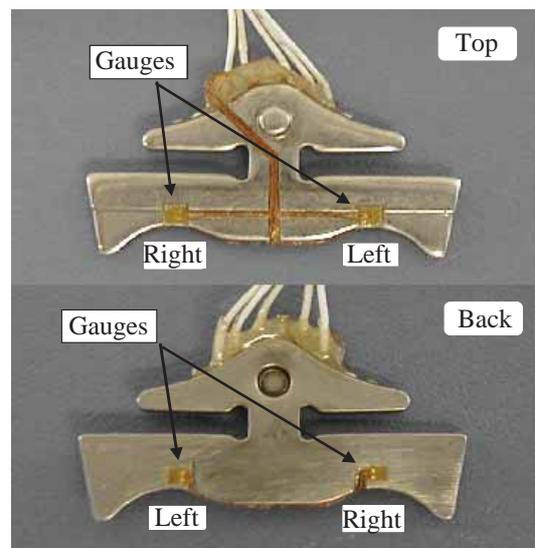
**Fig. 8** Width direction load sensor.
