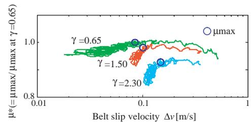
Fig. 13 Relation between slip velocity and belt  $\mu$ . ( $N_{in}$ =1000rpm,  $T_{in}$ =100Nm)
