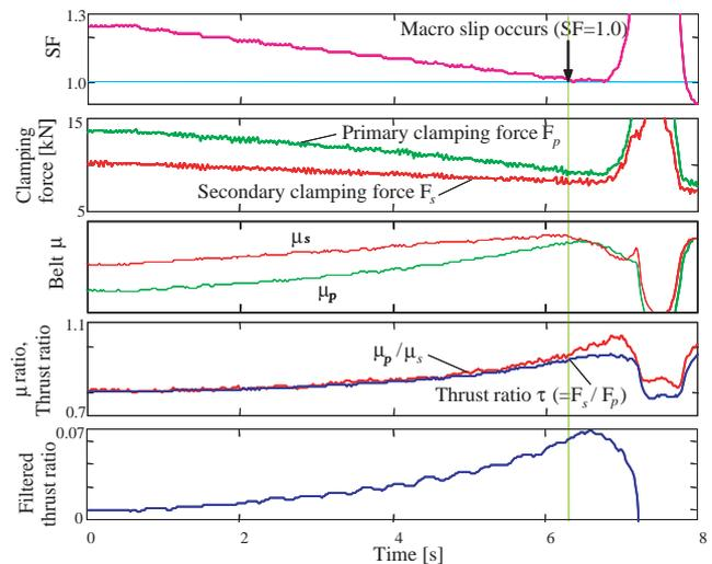
Fig. 19 Time chart of belt  $\mu$  and  $\mu$  ratio around macro slip occurrence. ( $N_{in}=1000\text{rpm}$ ,  $T_{in}=100\text{Nm}$ , speed ratio=1.0)
