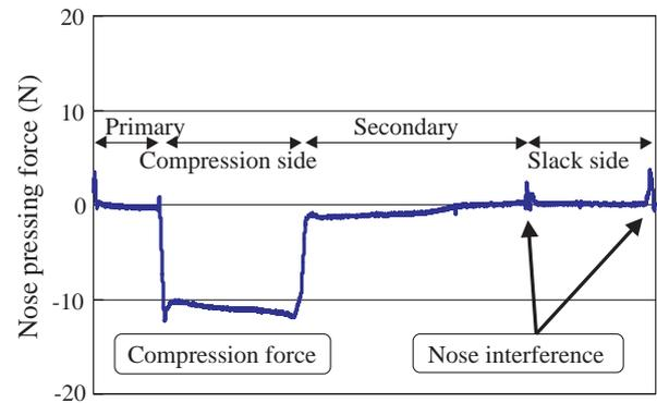
**Fig. 7** Measurement result of element nose strain. ( $N_{in}=500\text{rpm}$ ,  $T_{in}=150\text{Nm}$ , speed ratio=2.4)
