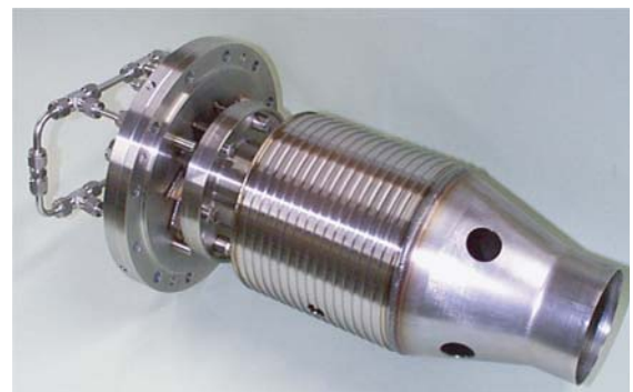
(b) Photograph of TLPP combustor.
