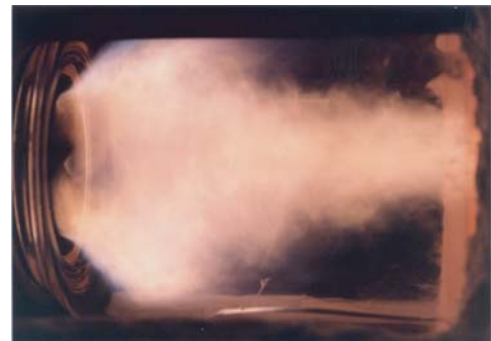
Fig. 5 (a) Spray combustion flame. (Using kerosene as the fuel)
