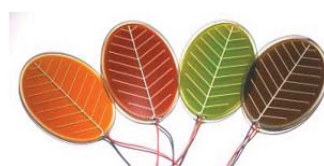
Fig. 3 Leaf-shaped transparent DSCs with four colors.
