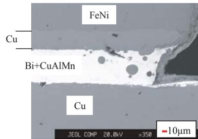
**Fig. 12** Cross sectional view of joint samples of Cu/FeNi/Cu chip and Cu/FeNi/Cu substrate after thermal cycling test of -40/250 °C, 200 cycles.
