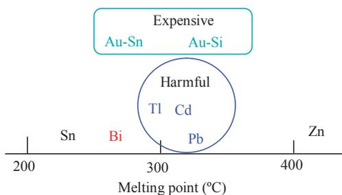
**Fig. 1** Overview of melting point of metals in the range from 200 to 450 °C.
