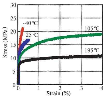
**Fig. 7** Temperature dependency of stress and strain properties of Bi+CuAlMn solder.
