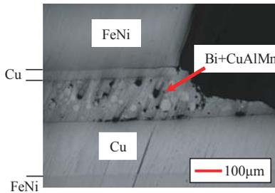
**Fig. 10** Cross sectional view of joint samples of Cu/FeNi/Cu chip and Cu/FeNi/Cu substrate after thermal cycling test of -40/200 °C, 1983 cycles.
