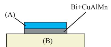
**Fig. 5** Illustration of a joint sample.
