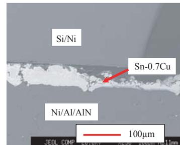
**Fig. 13** Cross sectional view of joint samples using conventional Sn-0.7Cu after thermal cycling test of -40/250 °C, 200 cycles.
