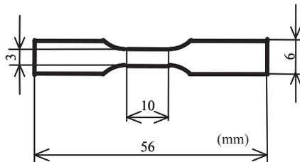
**Fig. 4** Schematic illustration of the test specimen. Thickness is 2 mm.
