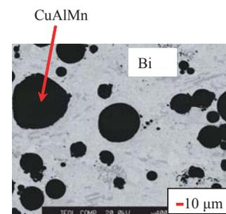
**Fig. 3** Cross sectional microstructure of the fabricated Bi+CuAlMn solder.
