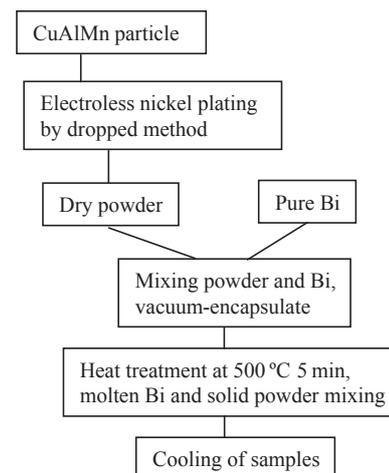
**Fig. 2** Fabrication process of Bi+CuAlMn solder.
