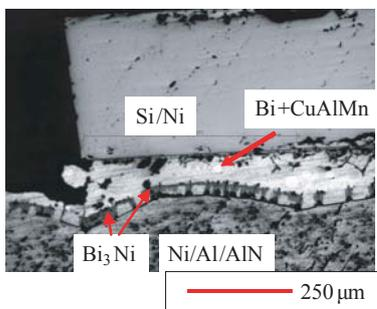
**Fig. 11** Cross sectional view of joint samples of Si/Ni chip and Ni/Al/AlN substrate after thermal cycling test of -40/200 °C, 1944 cycles.
