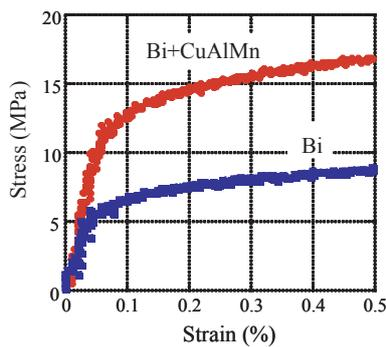
**Fig. 6** Stress and strain curve of solders comparison between Bi and Bi+CuAlMn solder at  $25\text{ }^{\circ}\text{C}$ .
