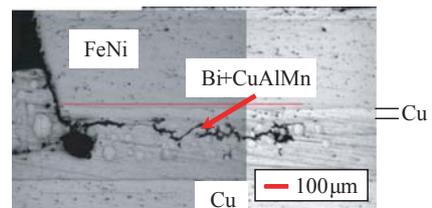
**Fig. 9** Cross sectional view of joint samples of Cu/FeNi/Cu chip and Cu substrate after thermal cycling test of  $-40/105\text{ }^{\circ}\text{C}$ , 200 cycles.
