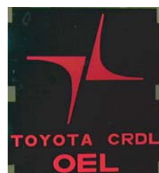
Fig. 4(c) Demonstration of a red phosphorescent OLED panel with Pt(II) porphyrin 4 .
