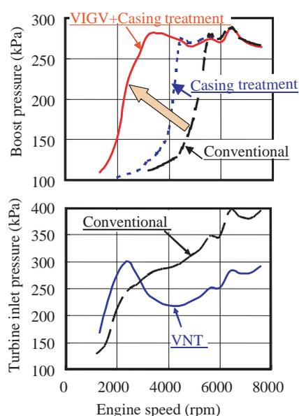
**Fig. 8** The effect of VIGV on the boost pressure.
