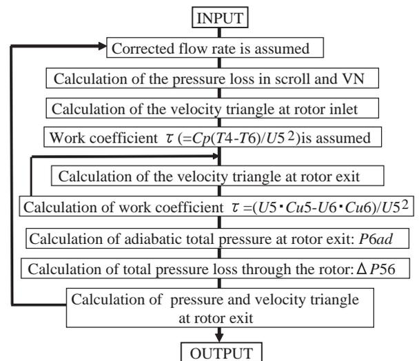
**Fig. 4** Calculation flow of the turbine model.
