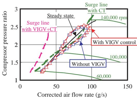
**Fig. 10** The operating line on the compressor map.
