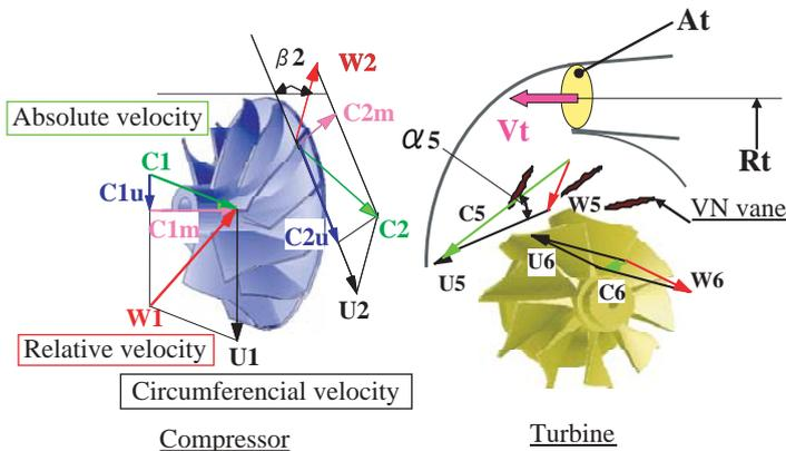
**Fig. 1** The velocity triangles of the compressor and turbine.
