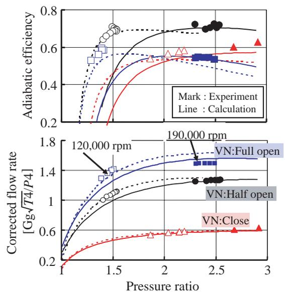
**Fig. 5** Comparison of the turbine performance between calculation and experiment.
