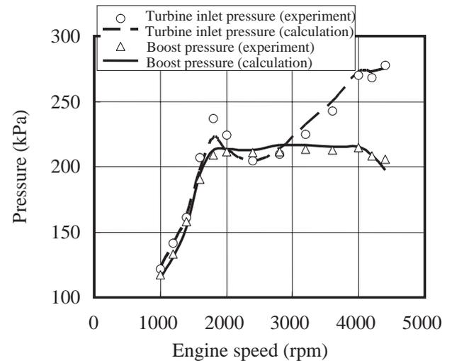
**Fig. 7** The predicted boost pressure and the back pressure compared with the experiment.
