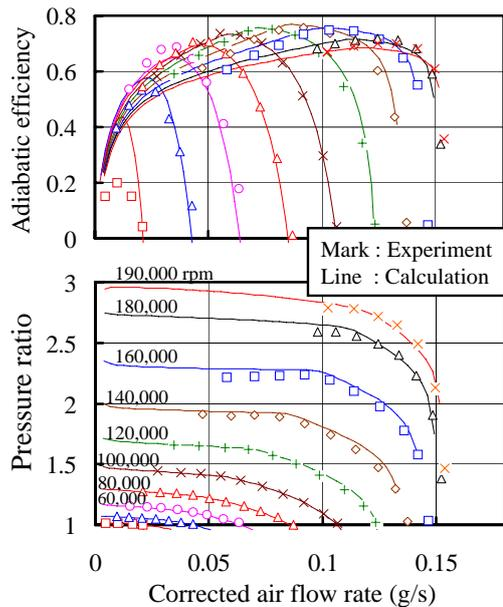
**Fig. 3** Comparison of the compressor performance between calculation and experiment.
