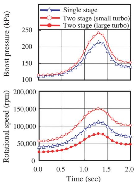
**Fig. 11** The transient response of the two-stage turbocharging system.
