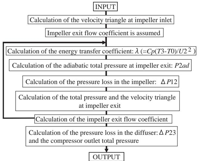
**Fig. 2** Calculation flow of the compressor model.
