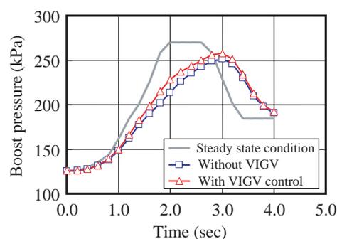
**Fig. 9** The effect of VIGV on the transient response.
