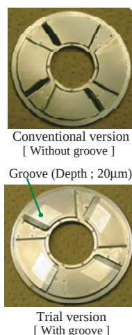
Fig. 4 Test pieces of compliant foil thrust bearing.
