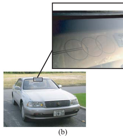
Fig. 10 Photograph of an antenna module. (a) Configuration of antenna module and (b) mounted antenna module on a windshield.
