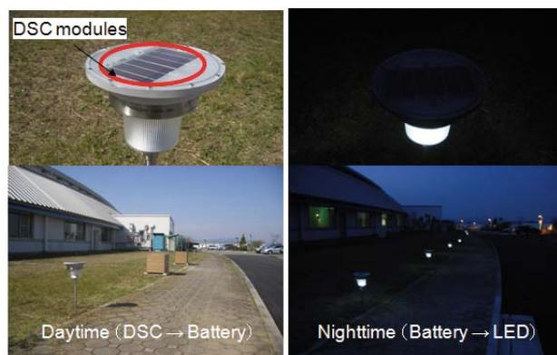
**Fig. 10** Solar-powered night-lights consisted of the DSC modules, the batteries and the white LED. They have been installed near the TOYOTA beam line of SPring-8, partly for the long-term outdoor test since May in 2009.
