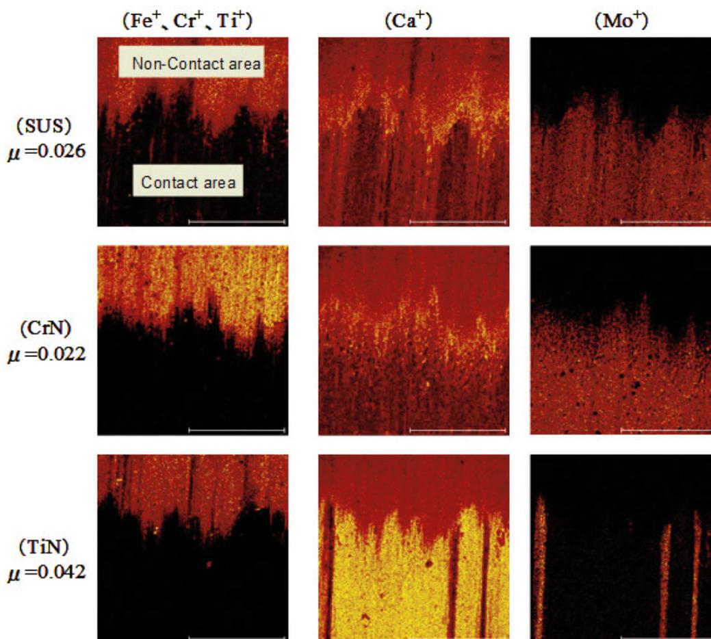
**Fig. 6** Positive ion images of the friction surfaces of three types of test blocks tested in engine oil B. The field of view is 200 square microns.
