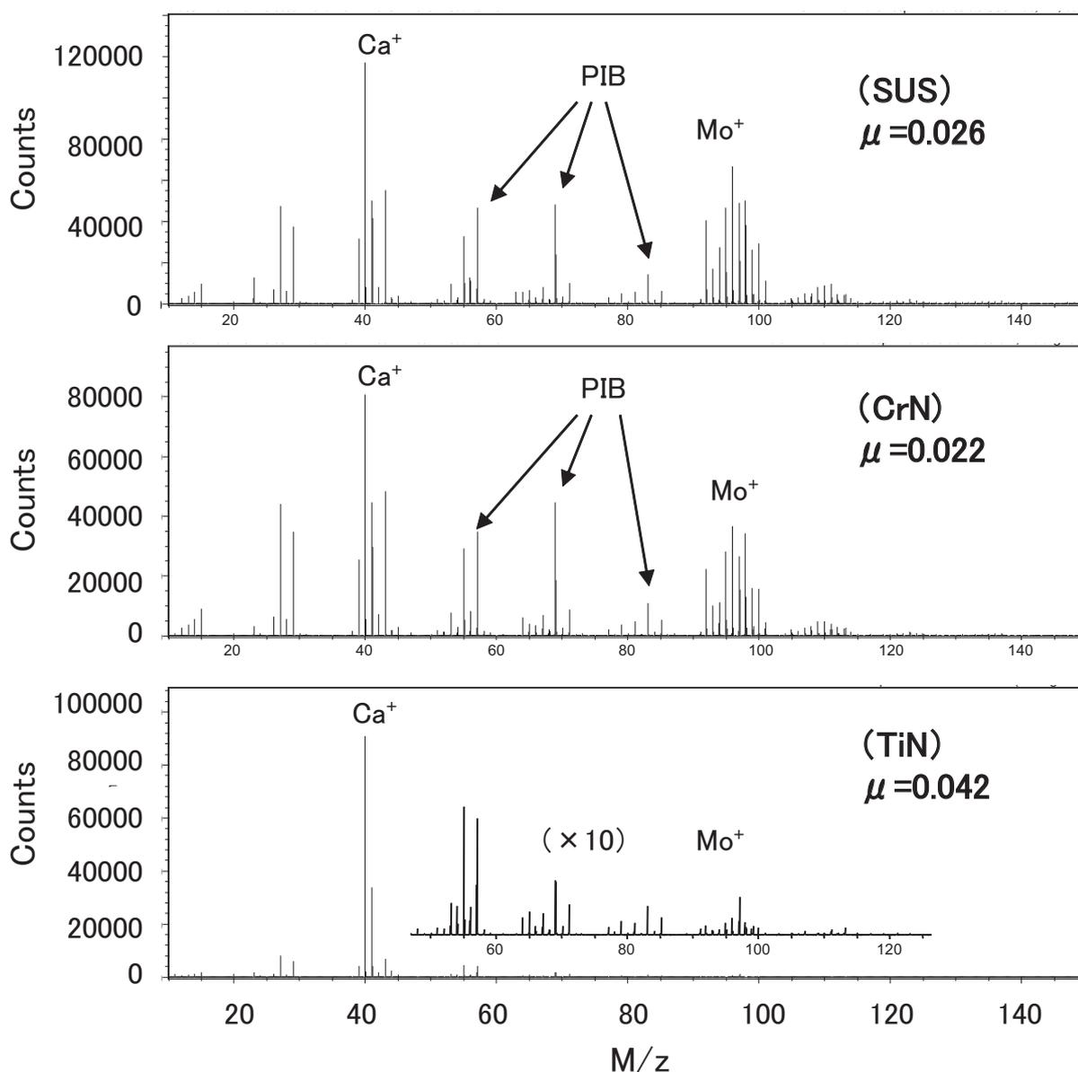
Fig. 5 Positive ion spectra of the friction surfaces of three types of test blocks tested in engine oil B.
