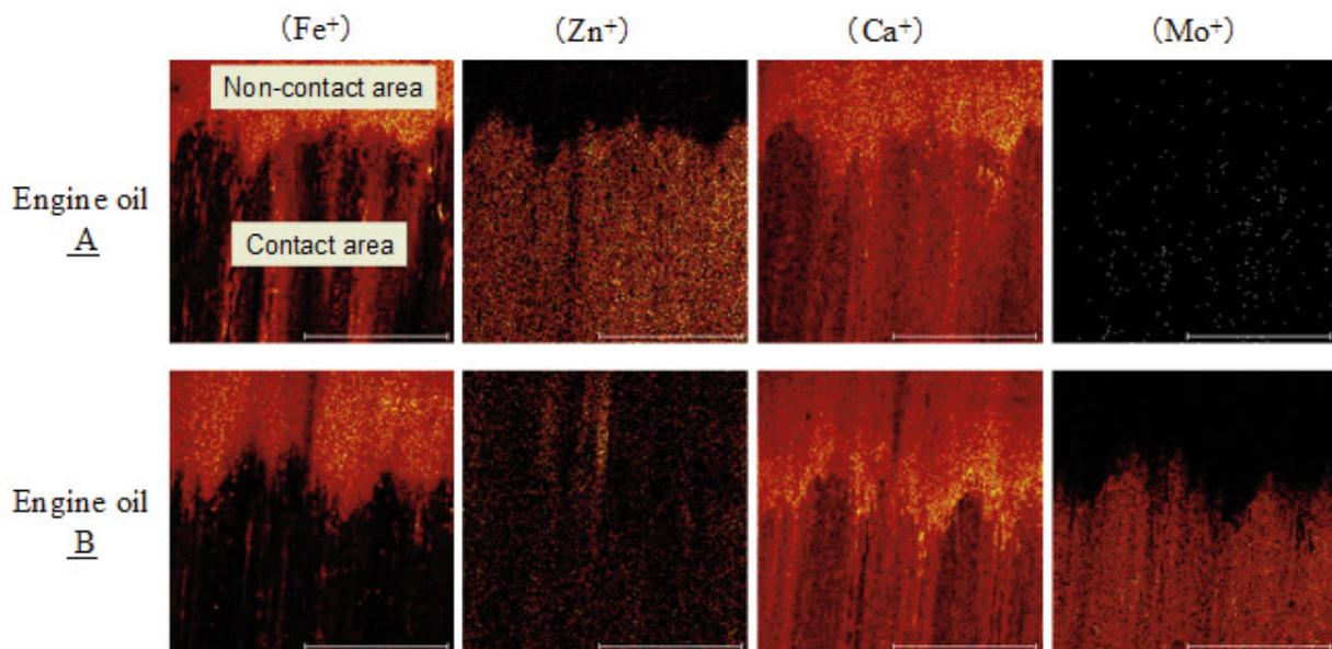
Fig. 4 Positive ion images of the friction surfaces of SUS test blocks tested in engine oils A and B. The field of view is 200 square microns.
