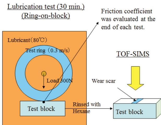
**Fig. 1** Schematic illustration of the lubrication test and preparation for TOF-SIMS analysis.
