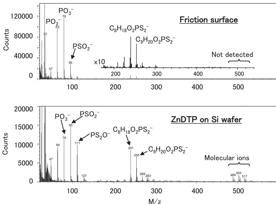
**Fig. 2** Negative ion spectra of the friction surface of SUS tested in a ZnDTP simple system (upper) and for ZnDTP on a silicon wafer (lower).
