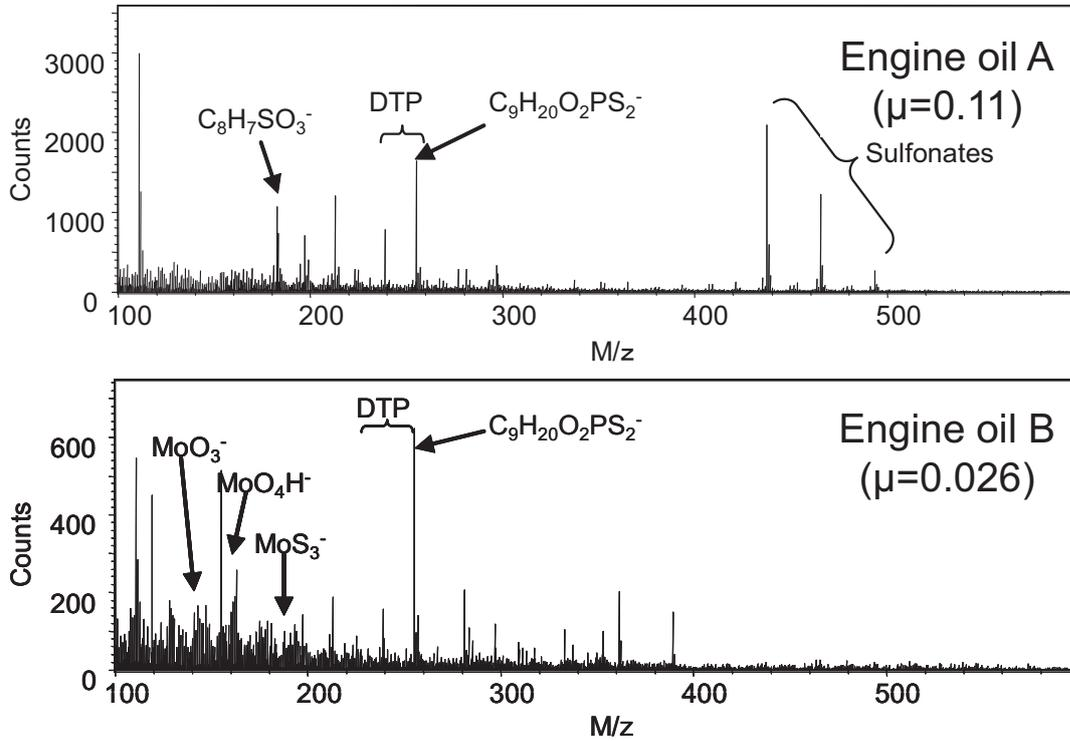
Fig. 3 Negative ion spectra of the friction surfaces of SUS test blocks, tested in engine oils A and B.
