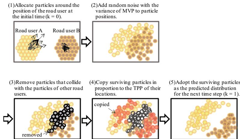
Fig. 5 Prediction procedure between different road users.
