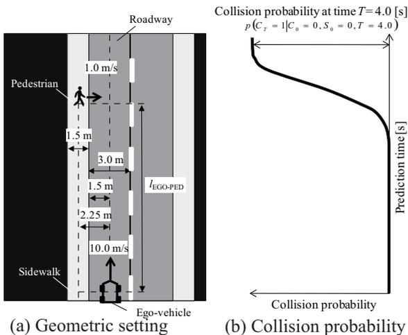
Fig. 6 Settings used in the numerical experiments.
