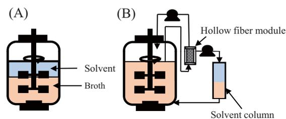
**Fig. 1** Schematic diagrams of extractive fermentation. (A) In situ extractive fermentation; (B) extractive fermentation with a hollow fiber module.
