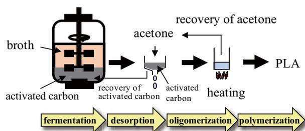
Fig. 10 Flow diagrams for Poly(lactic acid) (PLA) synthesis: from fermentation to polymerization.
