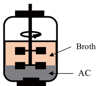
**Fig. 2** Schematic diagrams of adsorption fermentation.
