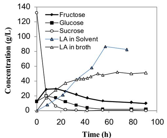
**Fig. 5** Extractive fermentation with a follow fiber module under pH 3.5 controlled condition.
