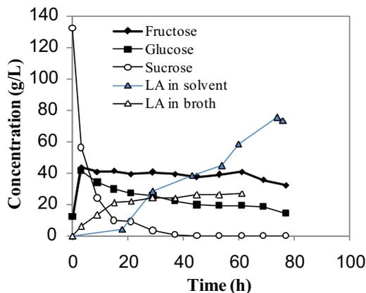
**Fig. 4** Extractive fermentation with a follow fiber module under pH-uncontrolled condition.
