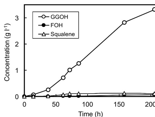
**Fig. 5** Fermentation profile of diploid prototroph strain 5X10 in a ten-liter jar-fermentor. After glucose feeding was stopped, as shown in the Materials and Methods, a mixed solution of glucose and ethanol (25% w/v and 50% v/v, respectively) was fed after 24 h at a feed rate of  $5.8 \text{ g h}^{-1}$ . The data represent the averages for duplicate samples.
