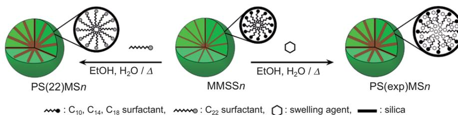
Fig. 4 Schematic representation of MMSS pore expansion.
