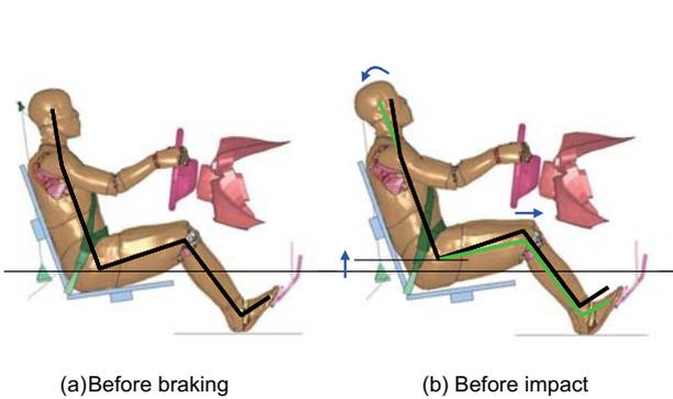
**Fig. 9** Comparison of driver's postures before braking motion and before impact.
