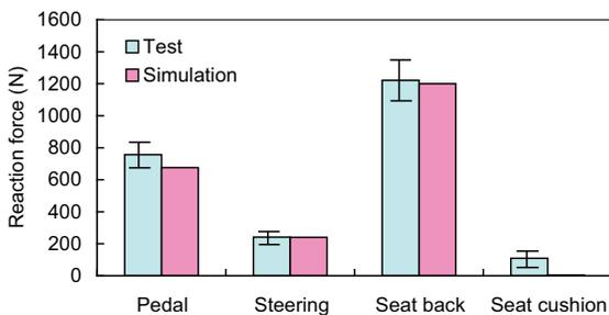
**Fig. 10** Comparison of reaction forces between simulation results and volunteer test data.
