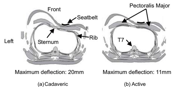
**Fig. 12** Comparison of the maximum rib deflection between cadaveric human model and active human model.
