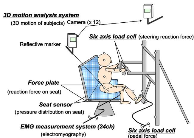
**Fig. 5** Diagram of developed measuring system.
