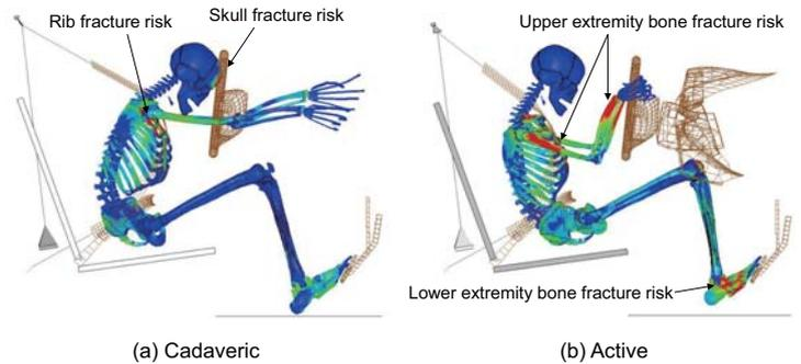
**Fig. 11** Comparison of stress distributions between cadaveric human model and active human model.
