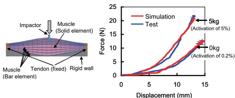
**Fig. 2** Force-displacement curves of an arm muscle.
